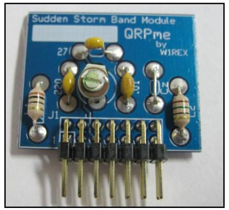
View of completed 40m band module board
