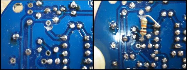
I solate the top pad for R4 then mount R4 to lower pad and IC pin. Now you can install resistor R4 on the bottom side of the board with one leg in the non-isolated hole and the other leg directly to pin 8 of the DIP socket.
