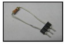
Crystal socket with resistor 'handle' Then I insert the socket into the board and
