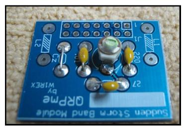
Band module board with caps installed.
