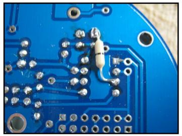
Back side view of completed SA612 ground mod
